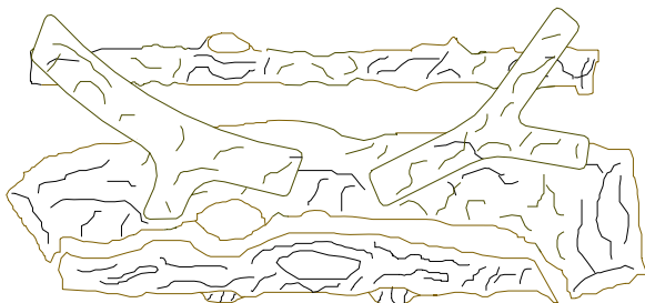
Figure 8A - Log Installation (270 Model)
